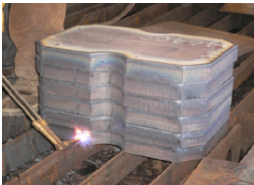
FIGURE 4. Manually post heating.
