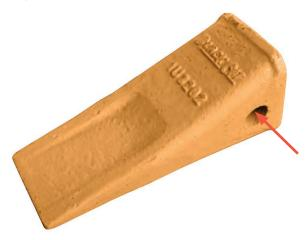
J-series has a pin and separate retainer. The pins have a recessed groove at one end to seat the retainer that is inserted into the adapter.
